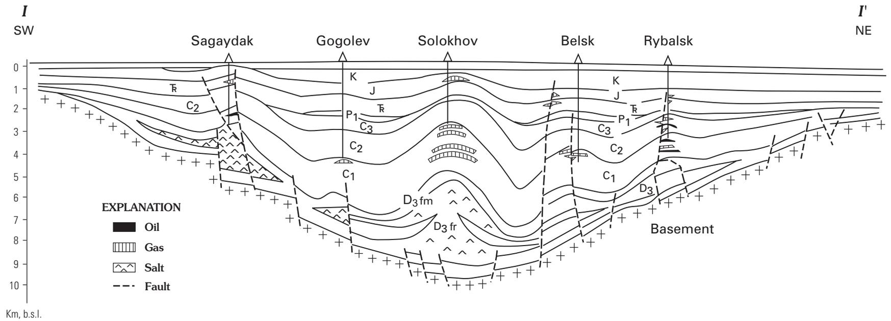
**Figure 4.** Cross section of Dnieper-Donets basin. Location is shown in figure 2. D<sub>3</sub>fr and D<sub>3</sub>fm are Frasnian and Famennian Stages, respectively, of the Upper Devonian; C<sub>1</sub>, C<sub>2</sub>, and C<sub>3</sub> are Lower, Middle, and Upper Carboniferous, respectively; P<sub>1</sub>, Lower Permian; R, Triassic; J, Jurassic; K, Cretaceous. Scale is not available. Approximate length of section is 160 km.
